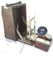
The shutter is not the usual Conley Safety or Wollensak Junior but the Wollensak Regno — a mechanical shutter with speeds from 1-100 T and B
